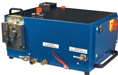
UNIPRESS 3: Universal machine for flaring and cutting ring pre-assembly
