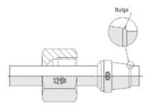
8. Insert the thus installed tube into the screw socket and tighten the union nut until there is a noticeable increase in force (pressure point). Afterwards screw in 30° - 60° with a suitable wrench. Hold the screw connection with a suitable wrench.
