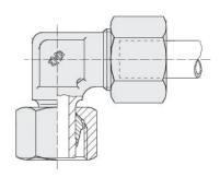
Oil the thread. Then insert the shaft into the screw connection and tighten with a wrench until there is a noticeable increase in force. For the final assembly of the shaft side, the union nut is tightened 30°-60° past the point of a noticeable increase in force.
