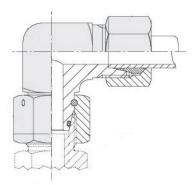
Oil the thread of the screw connection and O-shaped ring of the taper connection (DKO) side. Insert the taper couplings into a straight screw-in connection and tighten by hand. For the final assembly of the taper connection side, the union nut is tightened with 1/4 to 1/2 turns. The screw connection must be held using a suitable wrench.
